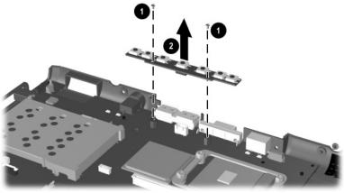
Removing the Switch Board
